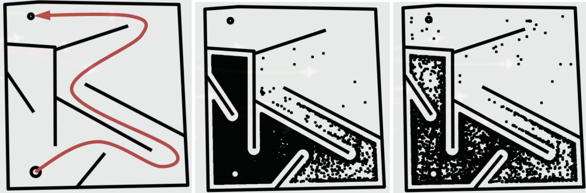
(a) The layout in the deceptive maze domain. (b) Final positions reached by the robot when directly minimizing the distance to the goal. (c) Final positions reached by the robot when applying diversity optimization (Novelty Search) to attempt to search for neural networks that reach every position in the maze. Notice that, despite ignoring the proximity of the robot to the goal location, more robots ends up finding the goal location.
